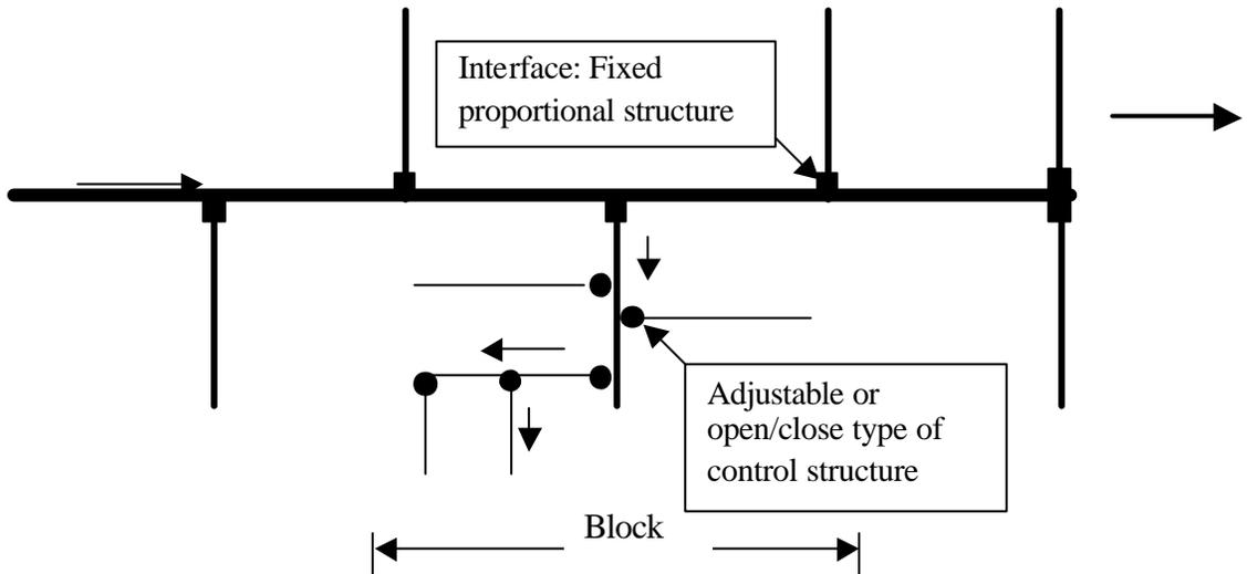
**Figure 3: Schematic Diagram of a Partially Proportionate System with Fixed Proportionate Section at Upper End**
