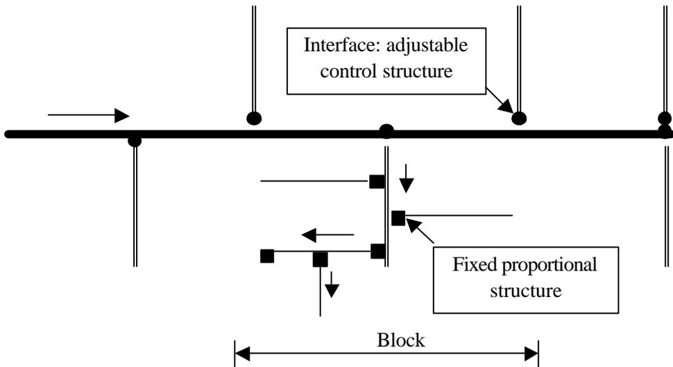
**Figure 1: Schematic Diagram of a Structured Irrigation System (Partially Proportionate System with Fixed Proportionate Section at Lower End)**
